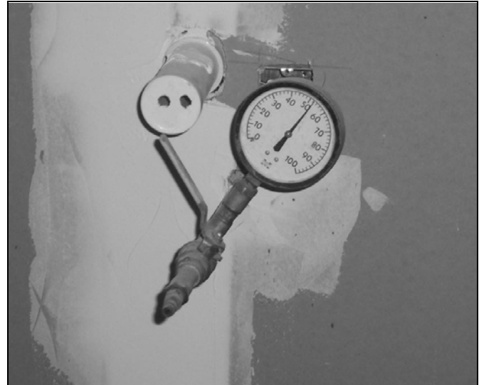
Figure P2503.9 IMPROPER GAUGE FOR TEST (DIAL INCREMENTS TOO LARGE)
